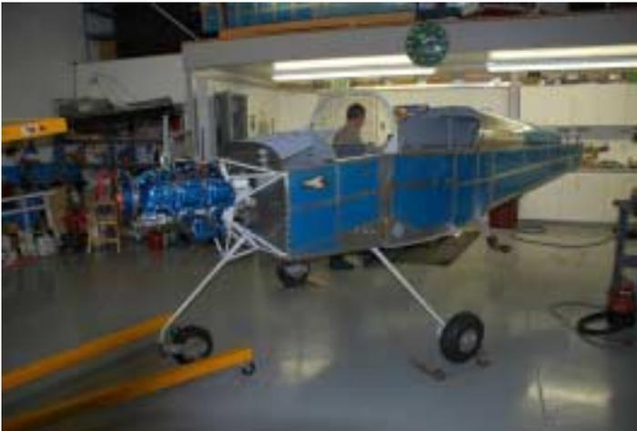
N619KB now has a motor. Installing it wasn't easy due to the FADEC fuel distributor block location on the top of the engine forcing the mounting loop to installed forward the engine which resulted in the engine being installed at a pretty good angle. Marv & I had to but the airplane on its tail in order to lift and angle the motor mount at the same angle as the engine. Getting the bottom bolts in were also a real pain!! Attached are some photos.
