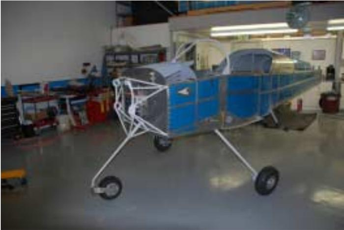
N619KB is now standing on its own set legs thanks to the help of Marv. Could have gotten the motor on last night as well, but had to do some reconfiguring on the MT prop gov to get the control arm going in the right direction for the RV setup. We should be able to get the motor installed during tonight's work session. Without the weight of the engine and wings, it stands really tall!!
