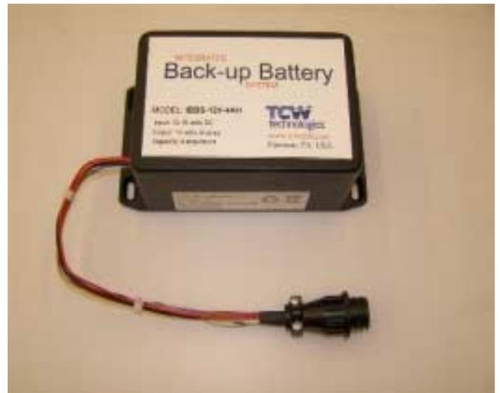
The *Integrated Back-up Battery System, IBBS*, is an electronic system that combines a Ni-mh battery pack, a charger and switching logic in one convenient package. The IBBS provides an engineered solution to enable an endurance bus for critical loads found in aircraft. It simplifies the wiring and installation of a source of back-up power by integrating all of the
