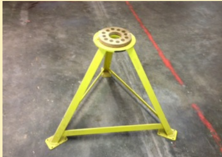
Engine Stand Prop Flange Interface for vertical mounting
