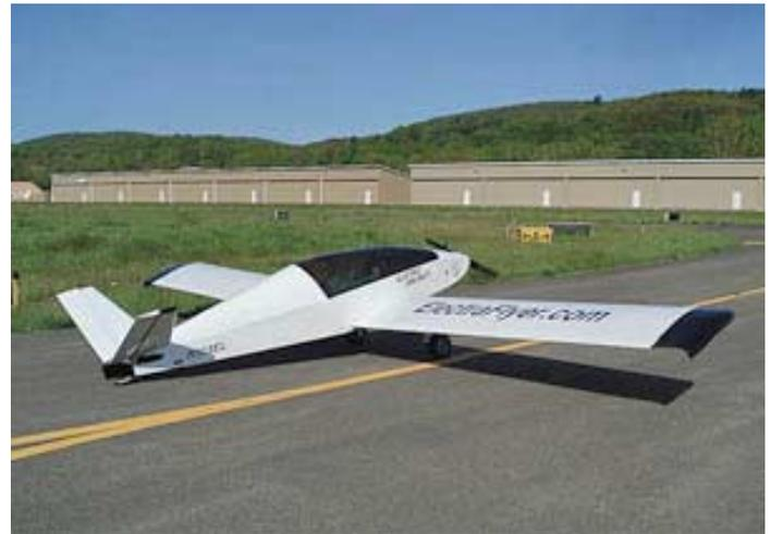
The ElectraFlyer-C, an electric-powered, single-seat airplane, recently made its first flight, reports Randall Fishman, president of Electric Aircraft Corp. Fishman previously flew an electric-powered weight-shift trike at EAA AirVenture Oshkosh 2007, for which he won grand champion ultralight and outstanding innovation awards. He is now using the same motor on an all-metal, low-wing airplane. He expects to demonstrate the ElectraFlyer C at AirVenture Oshkosh 2008.
